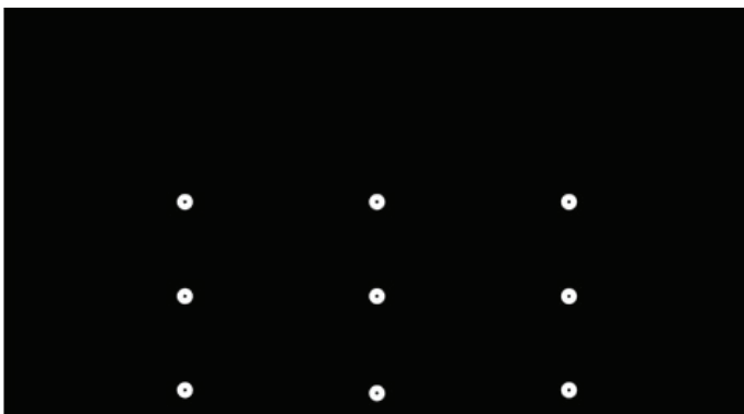
Figure 16. All stimulus points in the accuracy under ideal conditions test (Tobii T60 XL). The top left and right points are placed at a gaze angle of 20 degrees. The stimuli ratio corresponds to the screen resolution. The same stimuli are also used for the head position variation tests, as well as for the illumination dependent tests (barring the white background test).
