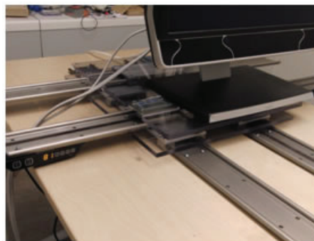
Figure 25. X-Y table. The X-Y table is designed to simplify the transition of head positions in the track box by moving the eye tracker to specific positions. The table is also vertically adjustable in order to accommodate all specified positions.
