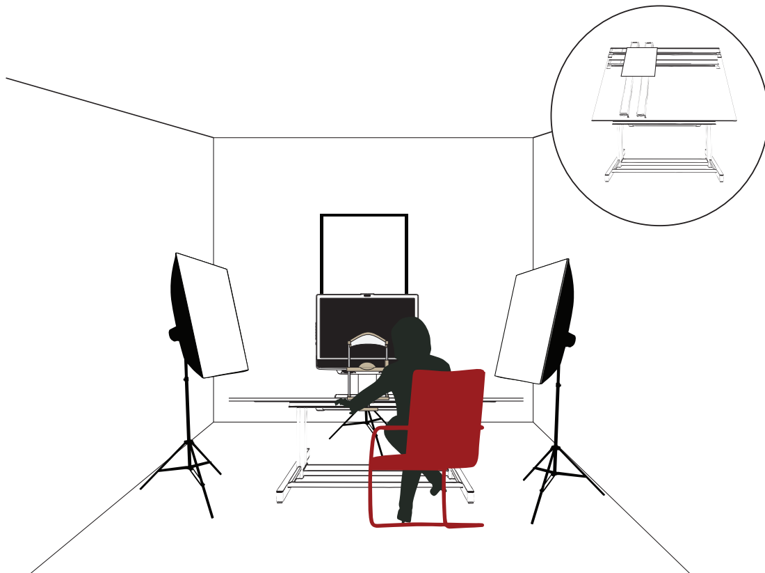
Figure 22. shows an illustration of a sample test environment. The eye tracker is placed on a X-Y table (detail, top right), with the test subject behind the chin rest. The room is illuminated by four soft boxes: two are placed on each side of the participant, one behind the eye tracker, and the fourth one is placed behind the participant facing the eye tracker. The fourth soft box is not shown in the illustration.
