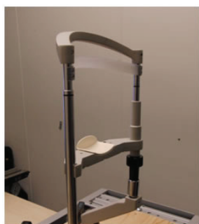
Figure 24. Chinrest. A chinrest is required in all tests to ensure the eye positions remain constant throughout the test series.
